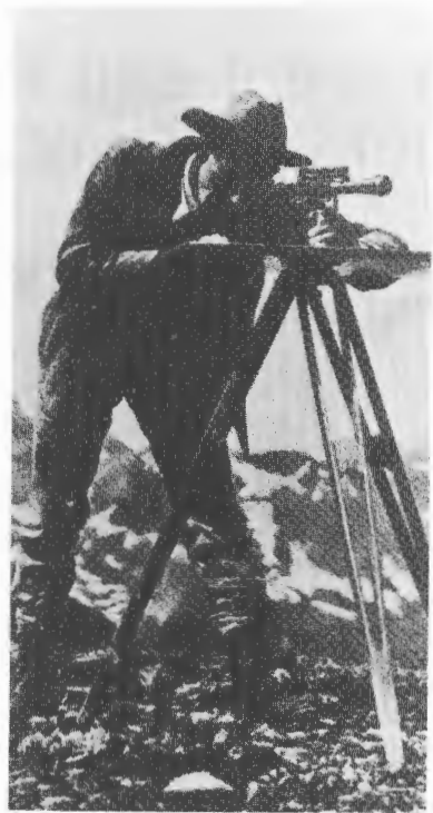
FIG. 2. Because it allowed drawing the map manuscript in the field, the plane table was considered by many to be the ultimate mapping instrument (U.S. Geological Survey).
